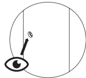
If screw is screwed into the tube, the arm is locked in the chosen direction.
