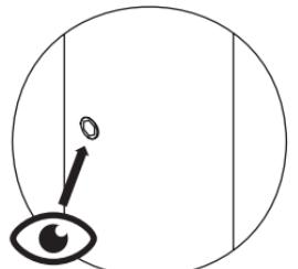
If screw is flushed with the surface, the arm can rotate freely.
