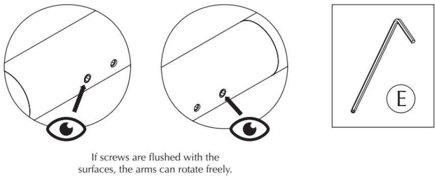
If screws are flushed with the surfaces, the arms can rotate freely.
