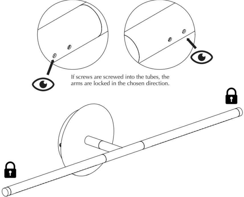
If screws are screwed into the tubes, the arms are locked in the chosen direction.
