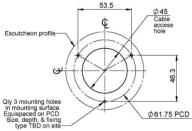
MOUNTING SEAT & ESCUTCHEON COVER Dimensions in mm
