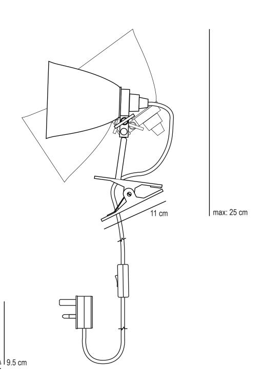
Use low energy CFL or LED candle/ball lamp for a combination of ambient and low level task lighting or R50 lamp if high level task illumination required.
